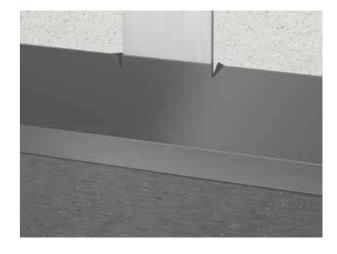
When installing Cembrit vertical profiles, it may be useful to cut and fold out a triangle on each side of the L profile, as shown in the illustration. This will prevent the horizontal profiles (Alu-L profile) from moving.
