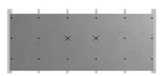
Example: Horizontally mounted boards with four intermediate aluminium profiles
