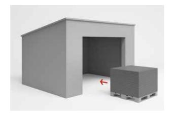
If Cembrit facade boards are stored more than 2-3 weeks on site, the pallets should be kept under a roof to ensure dry and ventilated conditions.
