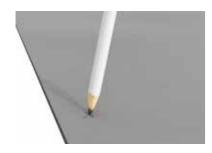
When marking the boards, make sure that marks are no larger than the hole to be drilled or no thicker than the blade that is to cut the board, as it can be difficult to remove marks from the board afterwards.
