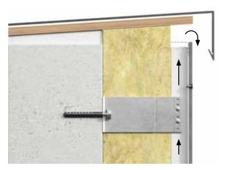
The passage of air must be maintained at the top of the facade whether it abuts to a roof or other structure. Just as at the base, there must be a ventilation gap of a minimum of 10mm or 100cm<sup>2</sup> per meter.
