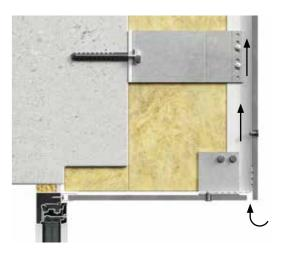
A horizontal free ventilation opening must be maintained above windows and doors as well. This ventilation gap must be at least 10mm wide. If steel, aluminium or plastic perforated profiles are used, a ventilation area opening of minimum 100cm<sup>2</sup> per meter is
