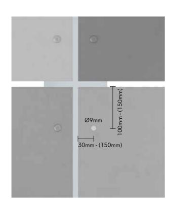
Example of vertical substructure
