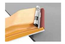
Once boards are cut, you can bevel the cut edge with a fine grinder (80 grain) to give the edge a pre-cut finish. The bevel should be angled at 45° relative to the board. This retains edge strength and removes small irregularities.
