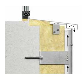
A horizontal ventilation opening of minimum 10mm or equivalent to 100cm<sup>2</sup> per meter should be maintained beneath windows or other openings where a sill is used. This ventilation gap is usually formed between the top edge of the facade boards and the bottom edge of the sill. It is recommended that the sill projects a minimum of 30mm beyond the front of the facade. This ensures that the water running from the sill does not enter the structure.
