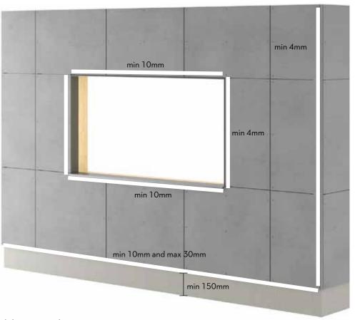
Make sure to follow the guidelines regarding distances described in this manual. The facade board should finish between 10 and 30mm below the bottom end of the substructure. For overhang and similar, the maximum distance is 100mm.
