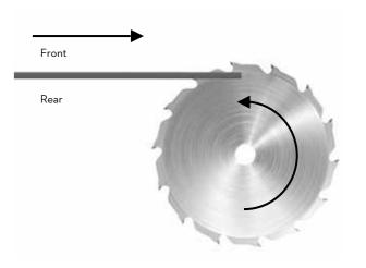
When using a table saw, place the board with the face uppermost on the table and cut from the rear of the board.
