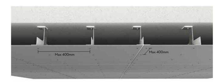
When using Cembrit facade boards as ceiling or soffit, you can normally use a regular aluminium system with brackets and T and L profiles, but for larger cavities, you need to contact an aluminium manufacturer to make sure the system fits your needs. The number of brackets and types of anchoring used for the type of deck/ceiling has to be calculated, and the manufacturer's instructions should always be followed.
