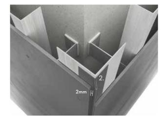
Cembrit External Corner Peak can also be used for  $90^{\circ}$  external corner constructions. It is installed in the same way as Cembrit External Corner Small. The distance from the inside edge of the facade boards to the profile should be a minimum of 2 mm.
