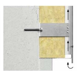
Air is pulled into the construction through an opening at the base of the facade, and it must be ensured that unobstructed ventilation is possible throughout the facade's height. There should be a ventilation gap of minimum 10mm, or equivalent 100cm<sup>2</sup> per meter. If perforated profiles are used, a ventilation area
