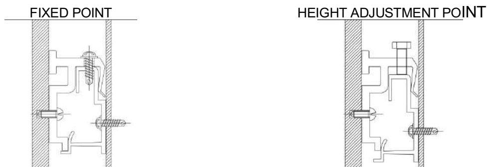
FIGURE 12: NATURCLAD-W HIDDEN FIXING KIT – FIXED POINT AND HEIGHT ADJUSTMENT POINT
