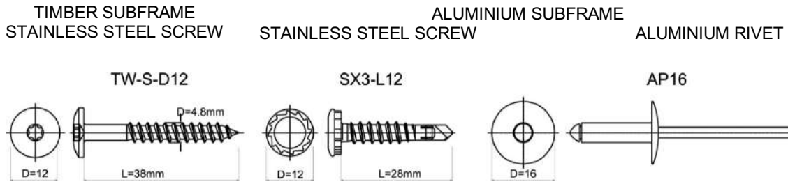
FIGURE 7: NATURCLAD-W EXPOSED FIXING KIT —CLADDING FIXINGS
